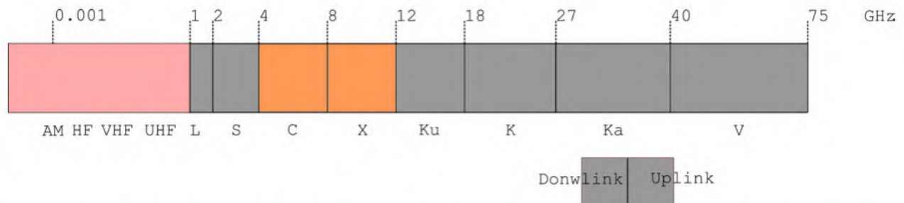
Figure 4.10: Mainly used in satellite communications. Terrestrial bands are red colored; satellite bands are in gray and shared bands in orange. Generally, the uplink is slightly above the downlink for satellite communications.
