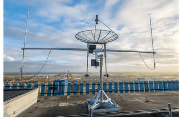
(b) Diameter of 3 m, gain of 31 dBi and a noise figure of 1.6 dB. Image retrieved from [57]
