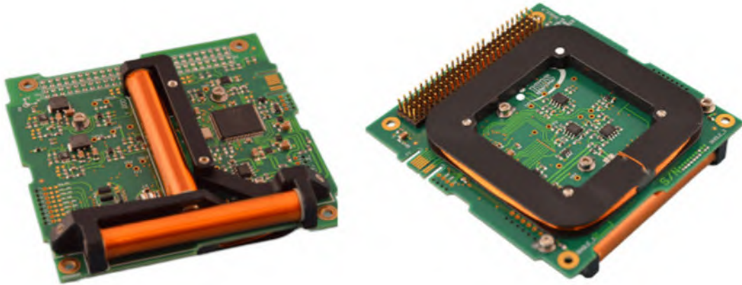
Figure 4.13: This magnetorquer PCB offers 3-axis magnetic actuation. Images retrieved from [49]
