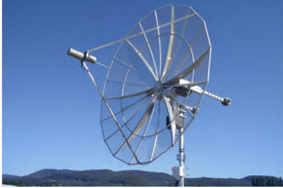
(a) Diameter of 3 m, gain of 35 dBi and a noise figure of 0.9 dB. Image retrieved from [56]
