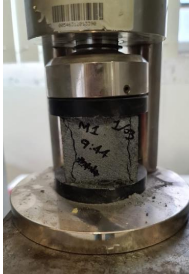
Figure 36. Compressive strength test of a casted sample
