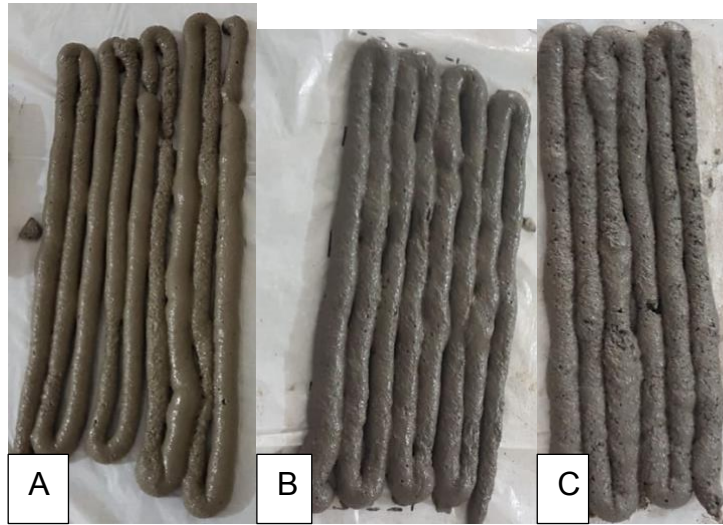
Figure 22. First layer extrusion of first round of preliminary tests (A) Test 1, (B) Test 3, (C) Test 7
