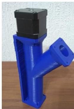
Figure 44. Second fabrication attempt of the extruder
