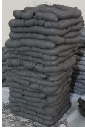
Figure 27. Buildability of Test 7.3 after 20 layers
