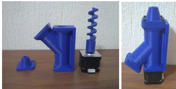
Figure 46. Fourth printing attempt of the extruder
