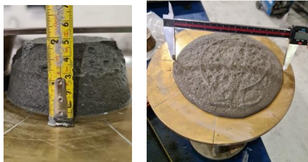
Figure 29. Slump test (left) and slump-flow test (right)
