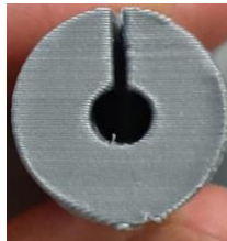
Figure 51. Hole in the screw for the motor shaft, second fabrication attempt of own design.
