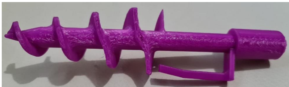
Figure 48. First fabrication attempt of the endless screw
