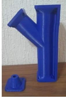
Figure 45. Third printing attempt of the extruder.
