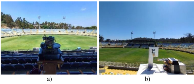
Fig. 1. 28 GHz radio system in the stadium Sausalito. a) Rx. b) Tx.
