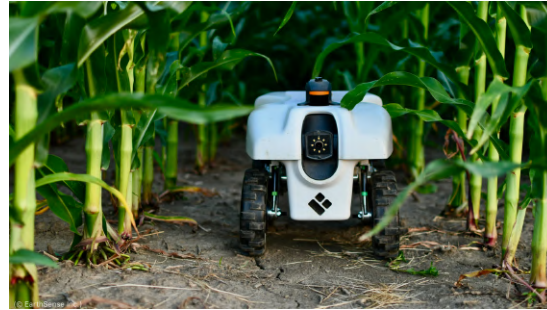
(c) A robot with sensors and a camera that travels the crop to collect information
