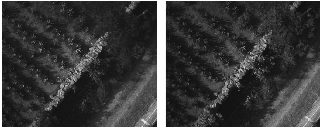
Figure 4.3: Channels blue and green in left and right respectively. The two images looks similar but they are not aligned. We can see a difference in the bottom-right corner in the wall
