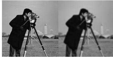
(a) Gaussian Filter. On the left side is the original image and the right side is the resultant to apply Gaussian filter, note that resultant image is fuzzy
