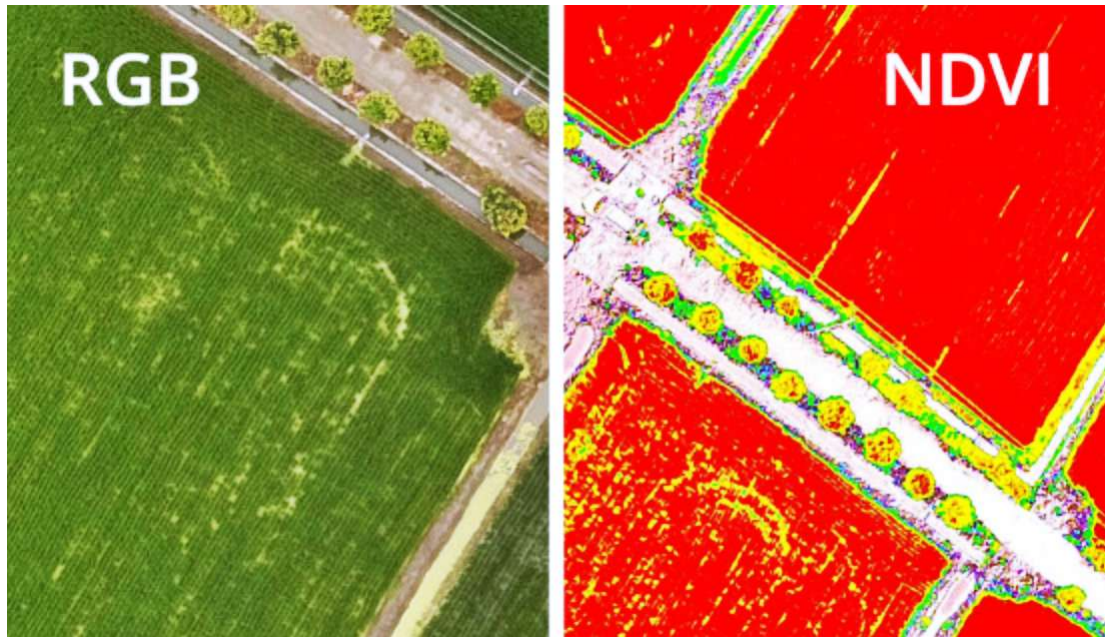
Figure 1.3: An example of an RGB image on the left and a NDVI image on the right
