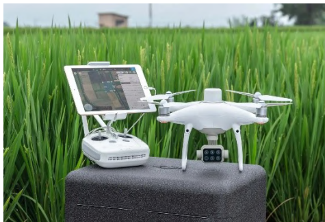
Figure 4.2: Drone P4 multispectral equipped with six cameras
