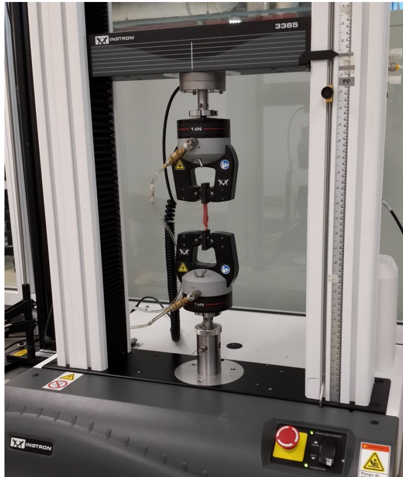
Fig. 89 Setup for Instron™ electromechanical universal testing system
