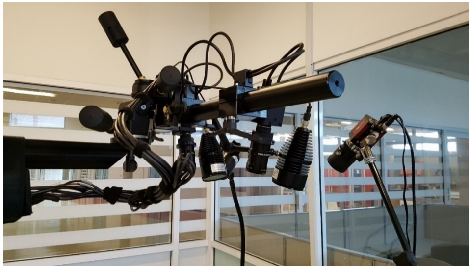
Fig. 97 GOM Aramis™ equipment set up for superficial deformation measurements based on image processing
