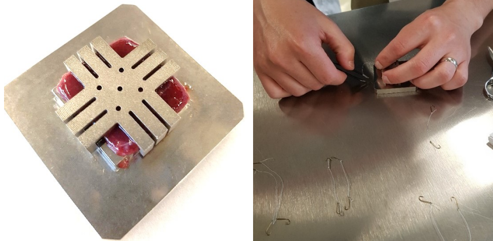
Fig. 100 Tooling provided to attach the fishhooks to the sample during preparation
