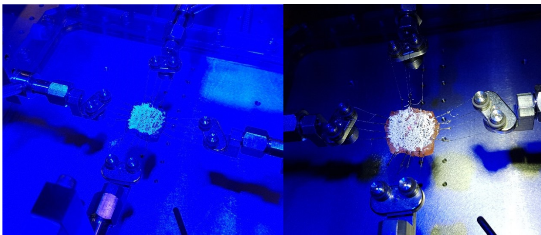
Fig. 102 Biaxial mechanical test set-up of porcine tissue samples
