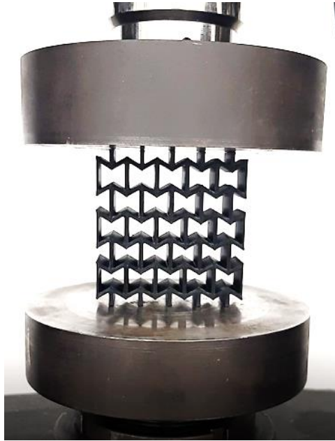
Figure 12. Set up for compressive test on PLA reentrant honeycomb samples.
