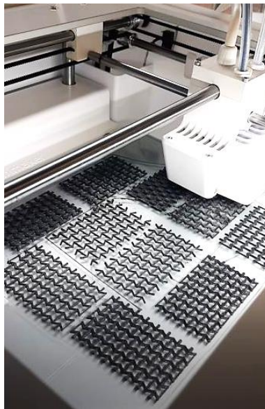
Figure 25. Printing process of reentrant honeycomb structures.
