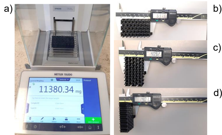
Figure 30. Measurement of relative density in printed specimens. The image shows the way of measuring a) mass, b) length, c) height, and d) depth of each sample.
