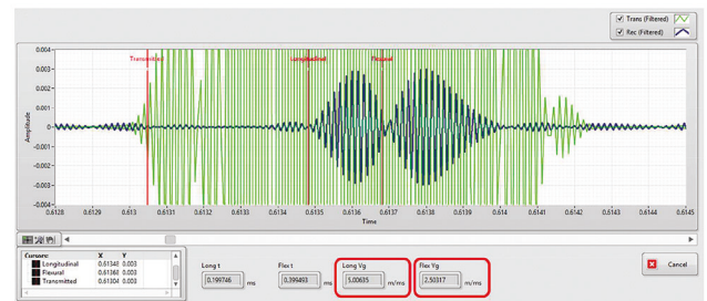
Figure 12. Acoustic propagation mode identification of a group of signals transmitted through 1 m of 1K22 MP-35N cable. The pale green curve shows the transmitted pulses and the dark green curve shows the excited guided wave modes
