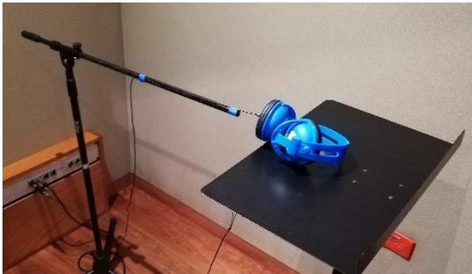
Fig. 16 ATVIO measured using MLS and inverse filtering technique. Headphones were measured inside an isolation booth to minimize sound reflection. Maximum Length Sequence method (MLS) reduces artifacts and noise signals recorded during the measurement.
