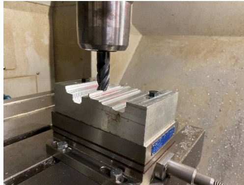
Figure 5.9 Experimental test to obtain the cutting forces
