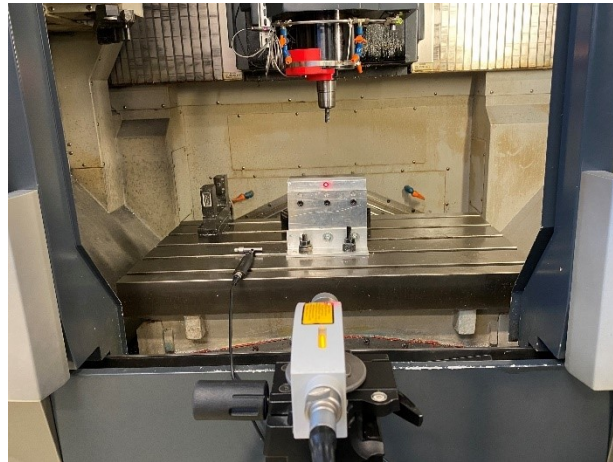
Figure 5.13 Experimental arrangement to characterize the milling tool
