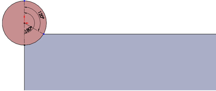
Figure 5.10 Scheme for the representation of \phi_{st} and \phi_{ex} for radial immersion of 25 %.
