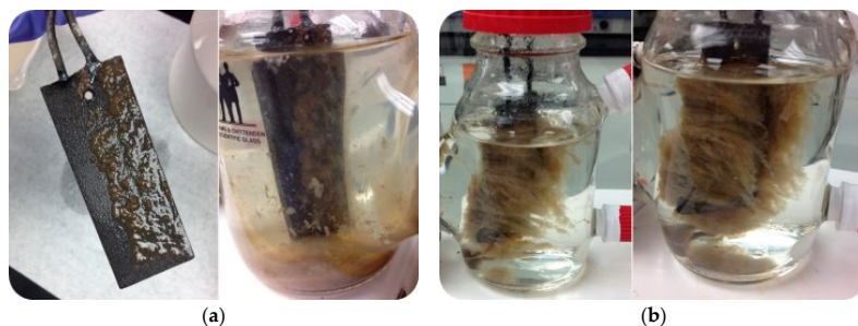
Figure 5. Differential growth and attachment of biomass on the electrode of the anode chamber. (a) Scenario NMC; (b) Scenario MC.
