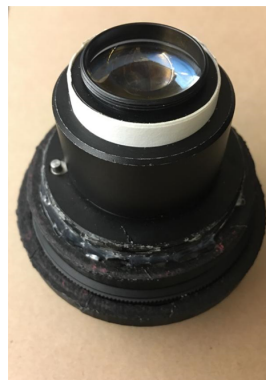
Figure 3.3: Lens used in the projector, assembled with a neutral filter.
