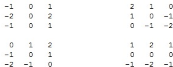
Figure 6.41: Convolution masks operator of Robinson
