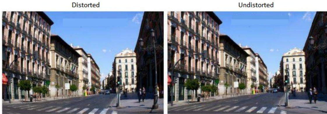
Figure 5.5: Radial distortion corrected
