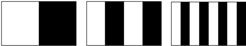
Figure 6.26: Reverse pattern of line R=2^0 R=2^1 R=2^2
