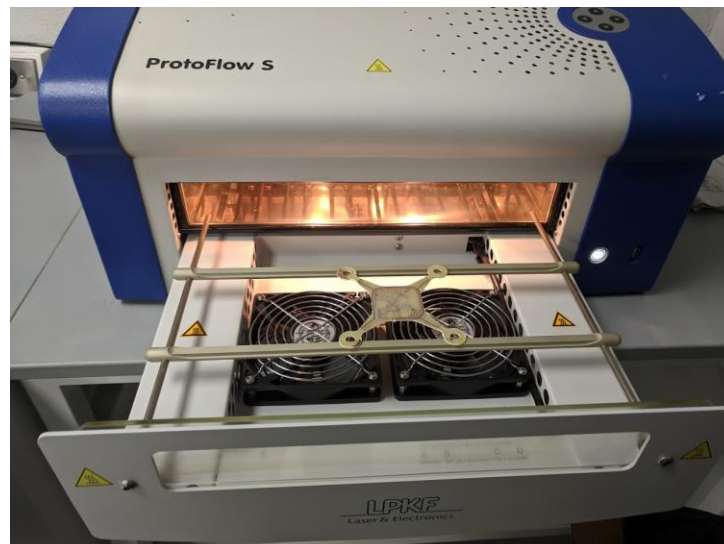
Figure B.7 Heat treatment of the ProConduct
