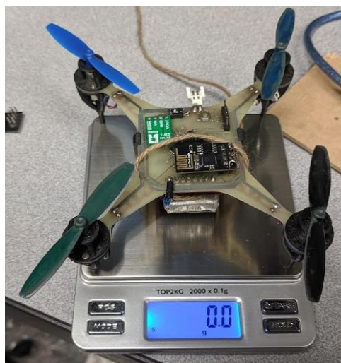
Figure 4.13 Testing setup to measure the force delivered by the motors
