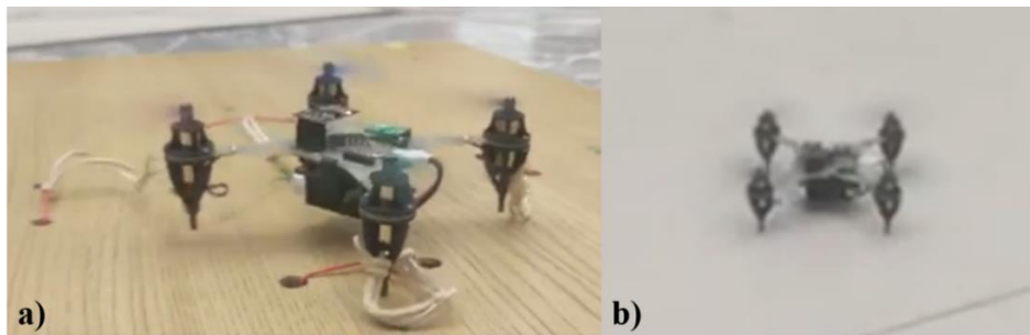
Figure 4.14 a) Drone anchored b) Drone free for final test
