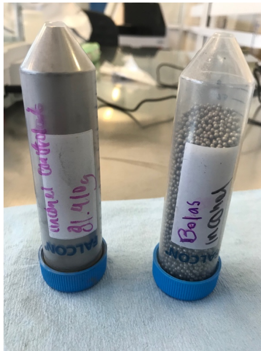
Fig 37 Weighted Inconel 718 and balls in closed containers.
