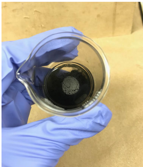
Fig 46 Phase differentiation between Inconel 718 and MWCNTs.
