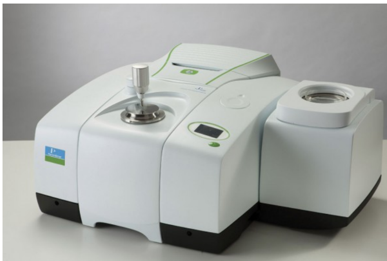
Figure 3.9: Equipment used for the vibrational bands found in the UHMWPE-TiO 2 nanocomposites. PerkinElmer Paragon 1000 FT-IR.
