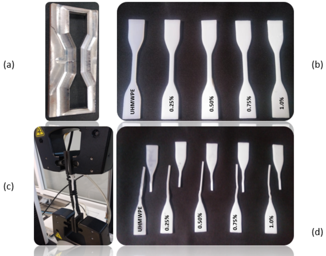
Figure 3.10: Tensile test arrangement: (a) Dog-bone sample cutter; (b) Representative batch of the dog-bone cut specimens based in ASTM D638; (c) Instron 336; (d) Representative sample result of the tensile tests per concentration.
