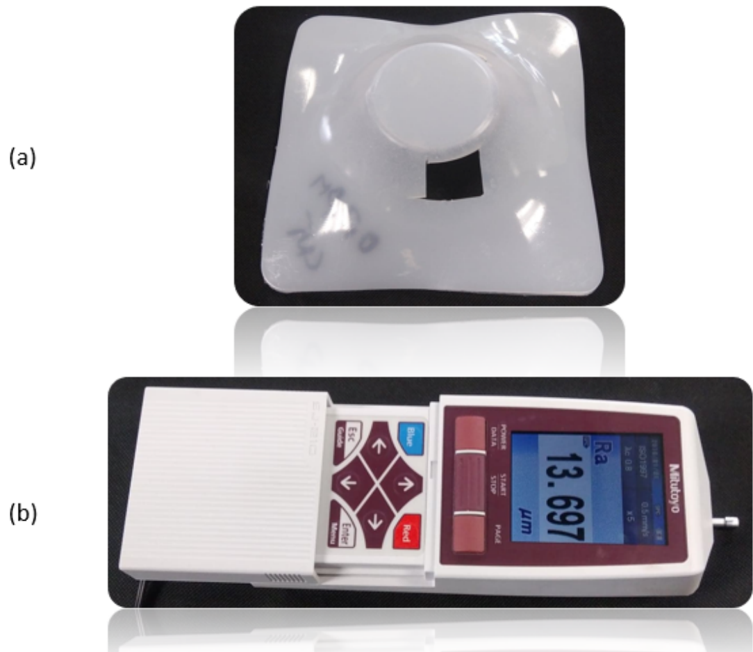
Figure 3.14: Roughness testing: (a) Partial section taken from UHMWPE-TiO 2 composites processed by SPIF for roughness analysis; (b) Mitutoyo SJ-210 profilometer equipment used for the study of superficial roughness.
