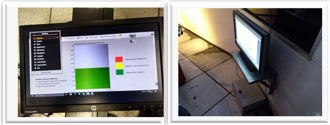
Fig 6.29 Screen that shows the risk indicator to the operator of the EAF
