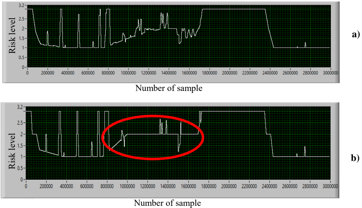
Fig. 5.17 Comparison between the out of the TSK model using triangular and trapezoidal MFs
