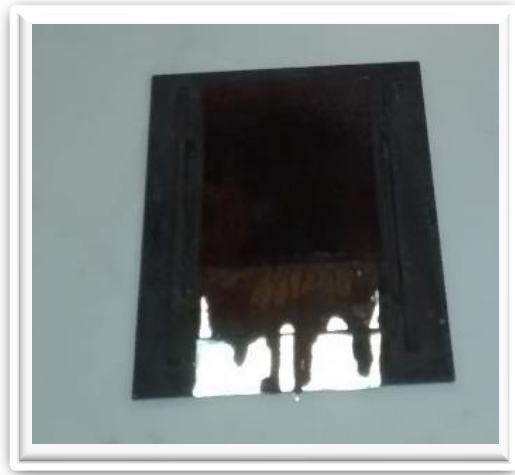
Fig. 4.18 Reflective material affected by high temperature
