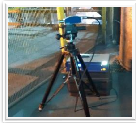
Fig. 4.2 Laser vibrometer at the steel shop
