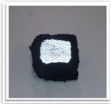
Fig. 4.19 Intact reflective surface after several days mounted at the EAF
