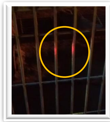
Fig. 4.17 Partial obstruction of the laser
