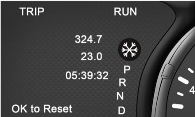
Figure 44 – Slippery Condition Warning
