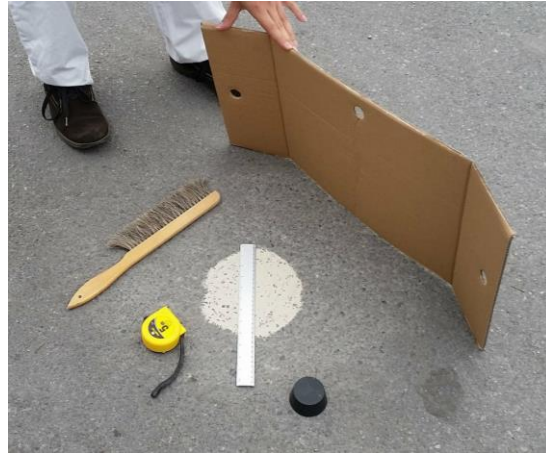
Figure 9 – Sand patch test (ASTM E 965)
