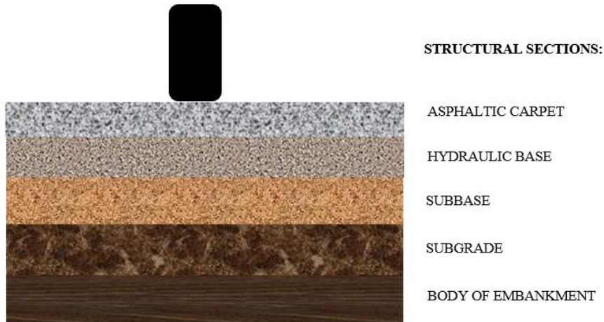
Figure 2 - Typical conformation of a flexible pavement.
