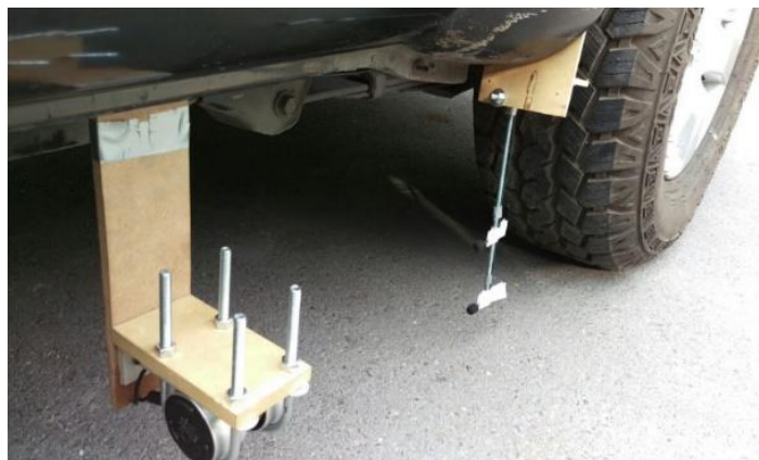
Figure 30 - Acoustic system mounted at the front of the driver's rear tire
