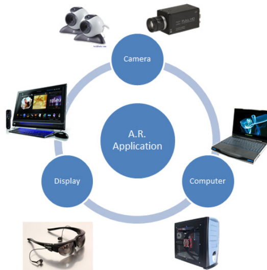
Fig. 4. Devices in an A.R. system Source: Carlos Castro, ITESM (2012)
