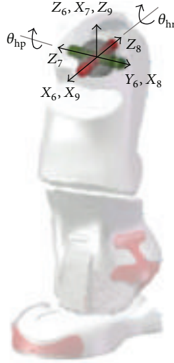
FIGURE 4: Forward orientation analysis of the humanoid leg.
