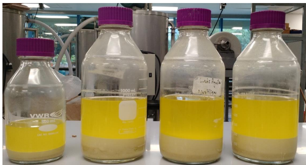
Figure 4.3 Fat Extraction of lupin's flour using Hexane.
