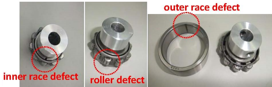
Figure 3.5: IR (left), RE (center), and OR (right) seeded defects [Wu et al., 2016]
