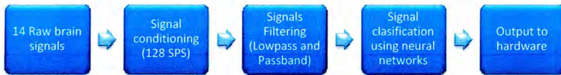
Figure 19. Structure for data analysis.
