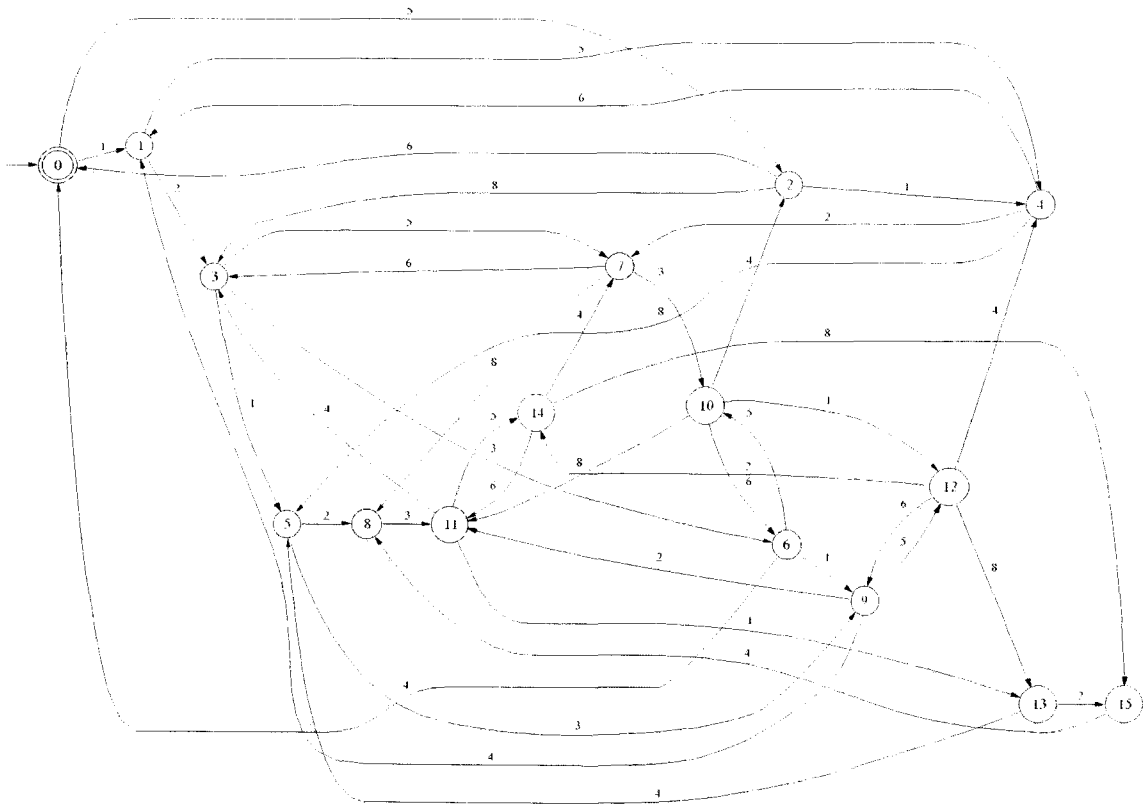
Figure 3.22: State-based representation for the first modular-agent for the case of B_1=2 .
