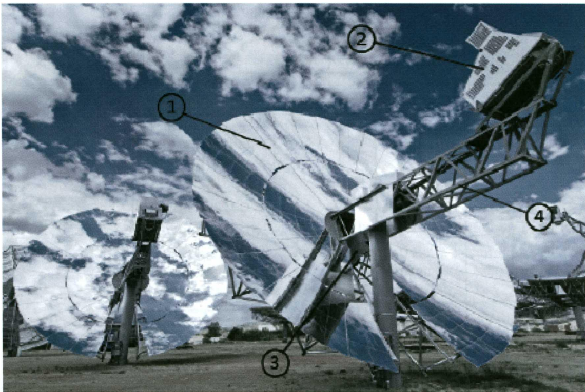
Figure 66: The main components of a typical solar concentrator are the parabolic concentrator (1), the receiver (2), the following system (3), and the supporting structure (4). The initial position of the tracking system should be calibrated to the particular position on the Earth's surface due to latitude variation.
