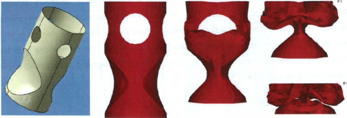
Figure 77: Deformation stages of the second concept. The relative simplicity makes simulations significantly shorter.
