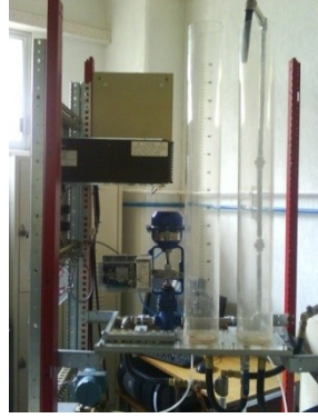
Figure A. 4. Physical Implementation of the Coupled-Tank System.
