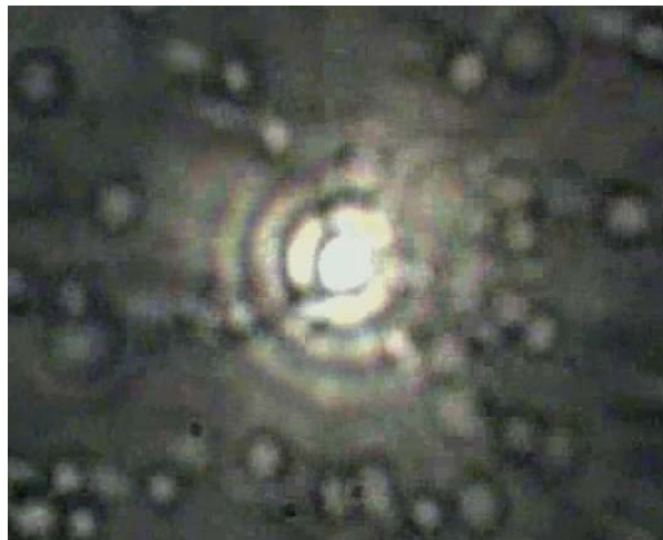
Figure 4.7: Transparent polystyrene particles 1.5 \mu\text{m} in diameter being trapped by a white light zeroth-order Bessel beam.
