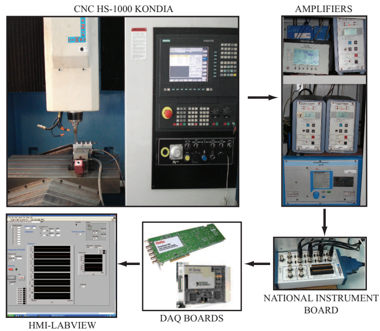
Figure 3.2: Experimental set-up: CNC machining center, amplifiers, DAQ boards, and LabView program.
