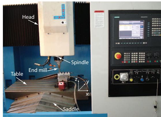
Figure 2.1: Main components and movements of the vertical milling machine
