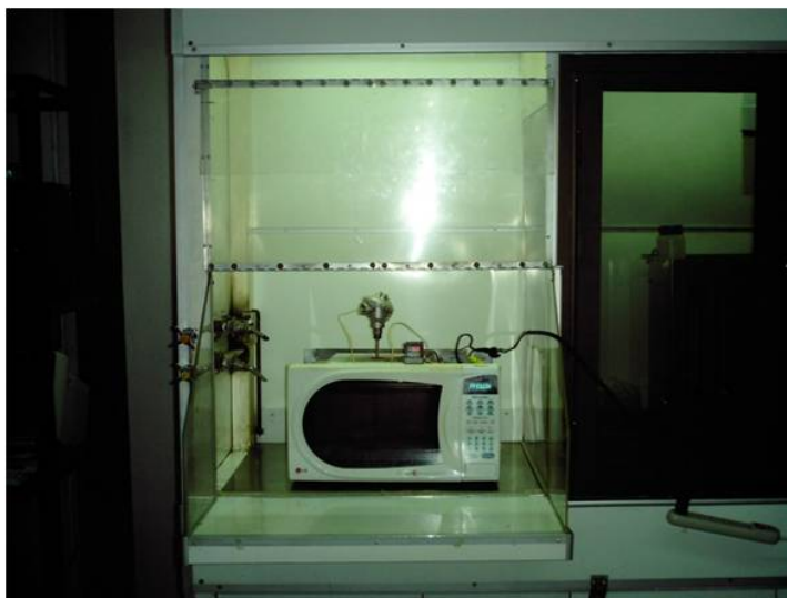
Figure 2.3 Microwave setup, temperature control is incorporated to the microwave unit to keep a constant temperature of the chemical bath.
