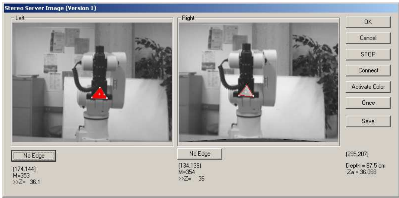
Figure C.4: Stereo images used for the learning process. For calibration purposes the left image is used as a reference while the right image is adjusted, this is observed by the curvature on the bottom.
