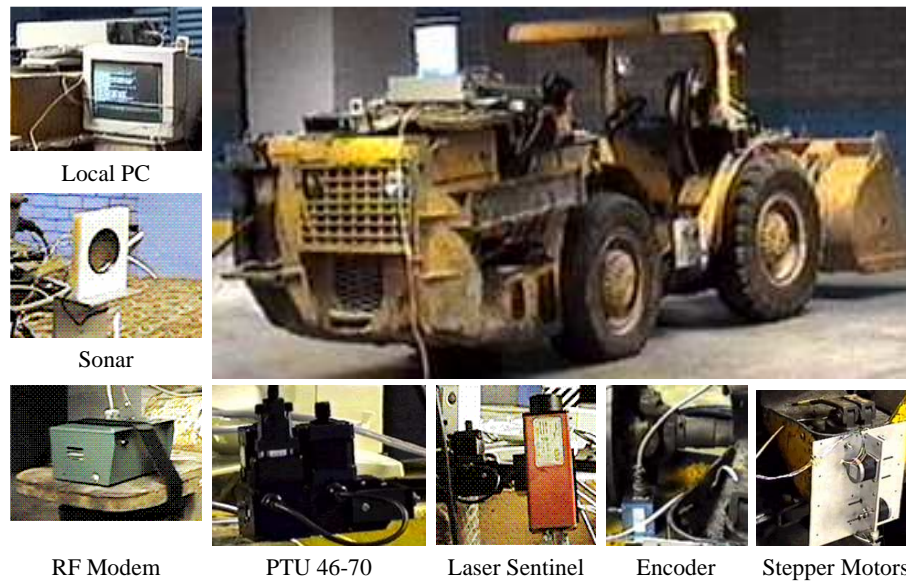
Figure 5.12: MAV prototype that integrates the components of the MAV configuration to perform the tunnel-profiling task.
