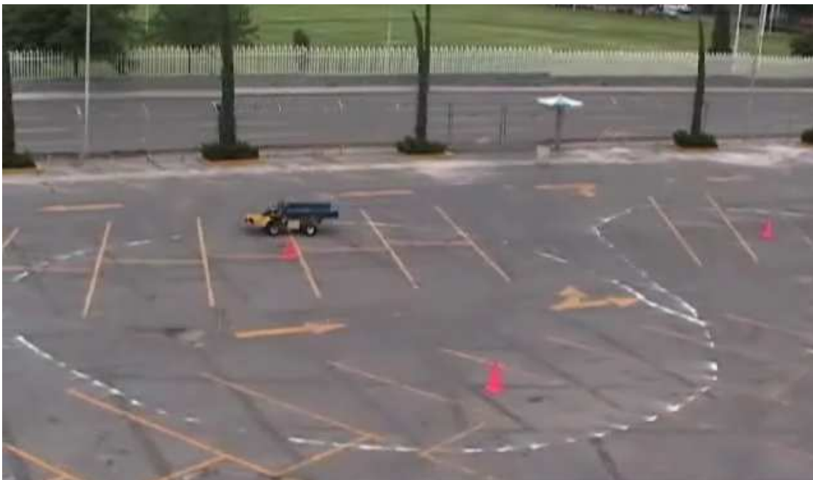
Figure 8.4: The robotic vehicle prototype while following a closed path to check the performance of the drive and steering controllers.
