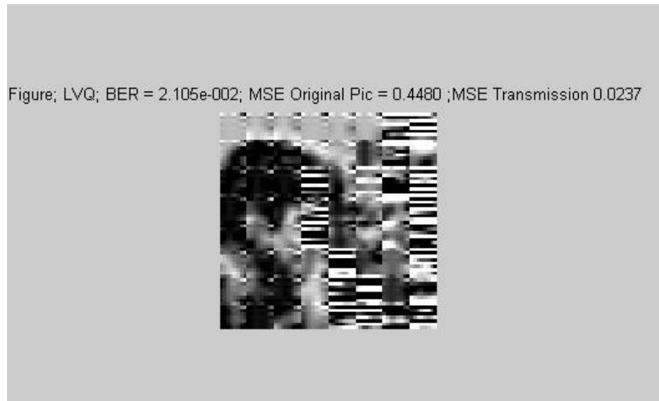
Figure A.3: E_B/N_0=2 dB Using LVQ Quantization
