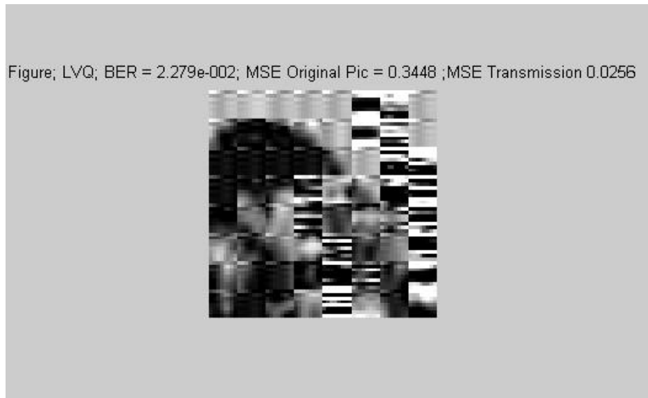
Figure A.5: E_B/N_0=3 dB Using LVQ Quantization
