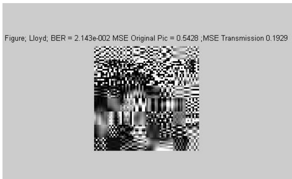
Figure A.6: E_B/N_0=3 dB Using Lloyds Quantization
