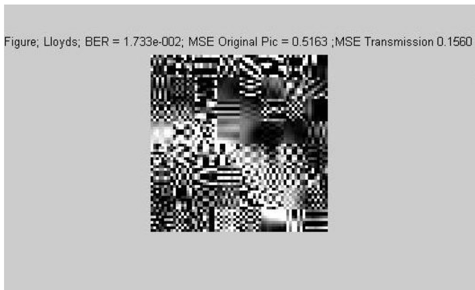
Figure 5.12: E_B/N_0=3 dB Using Lloyds Quantization
