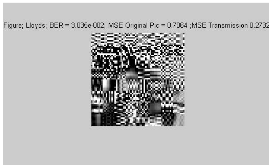
Figure A.4: E_B/N_0=2 dB Using Lloyds Quantization
