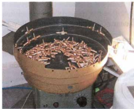
Figure 4.9: Vibratory bowl feeder with active sensing reorientation.
