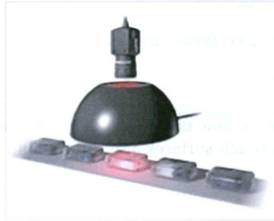
Figure 2.17: Diffuse On-Axis lighting
