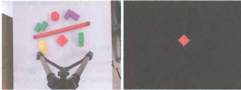
Figure 5.11: RGB image (left) and Input image(right) for red pieces
