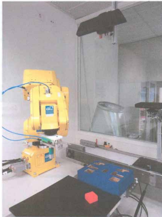
Figure 5.51: Acquisition of 3D data of one object
