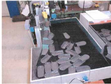
Figure 4.8: Vibratory brush feeder for gentle feeding of fragile parts.
