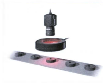
Figure 2.7: Direct front lighting
