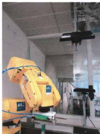
Figure 5.29: Camera Mounting Implementation
