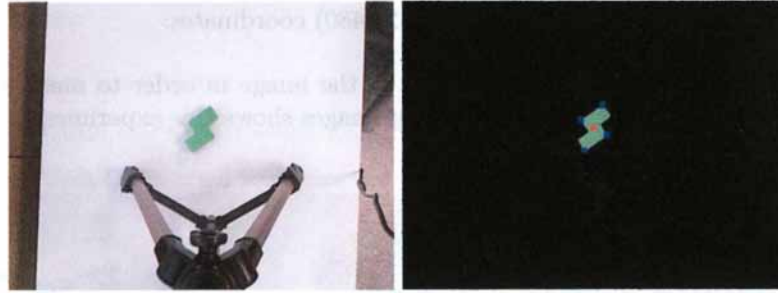
Figure 5.17: RGB image(left) and input image(right) for green pieces
