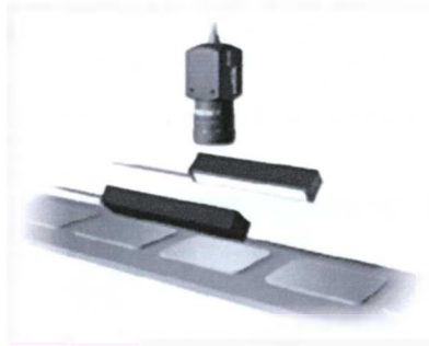
Figure 2.15: Dark field lighting
