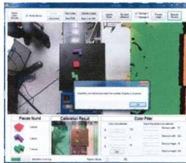
Figure 5.58: Interface behavior when the number or type of pieces are not correct for the package requested
