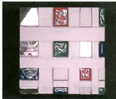
Figure 2.18: Diffuse On-Axis lighting application
