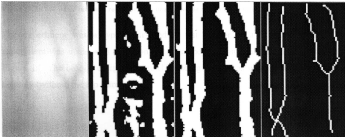
Figure 12. Black & white, filtering and thinning steps for finger-vein image recognition (Cheng-Bo, 2009)
