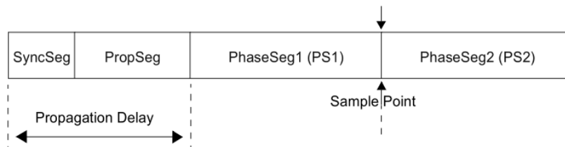
Figure 2-20: Nominal bit time segments as defined by Microchip [Microchip, 2007].
