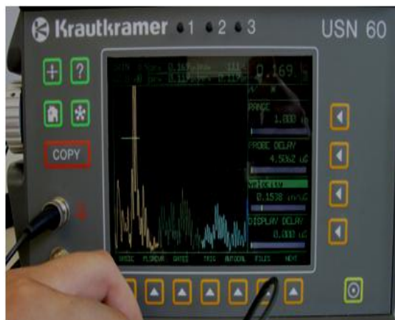
Figure 35 Shear beam detection
