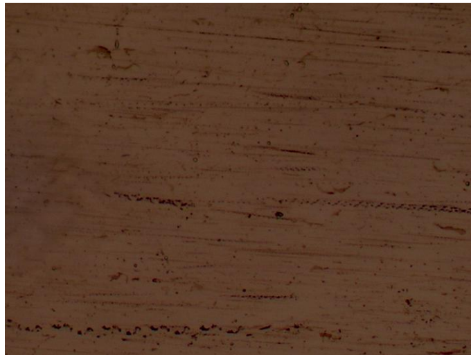
Figure 23 Microstructural aluminium 3003 HAZ as polish 100x
