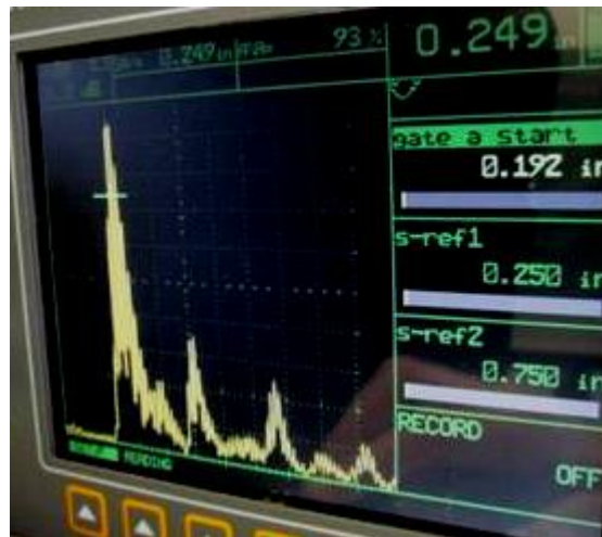
Figure 50 Autocal submenu of kraufkramer for first reference
