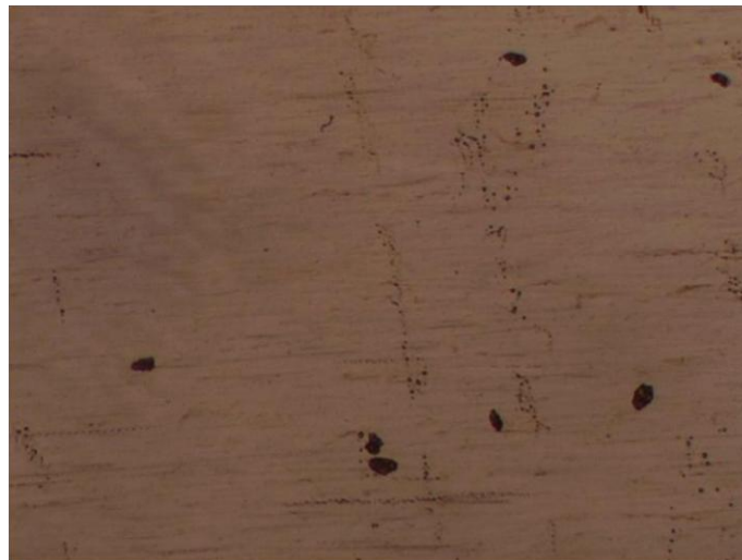
Figure 21 Microstructure aluminium 3003 SZ and TMAZ as polish 50x
