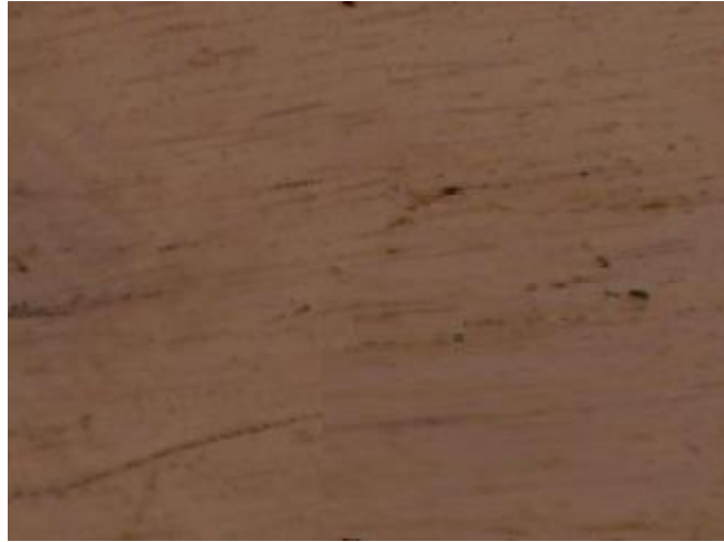
Figure 22 Microstructural aluminium 3003 SZ as polish 100x
