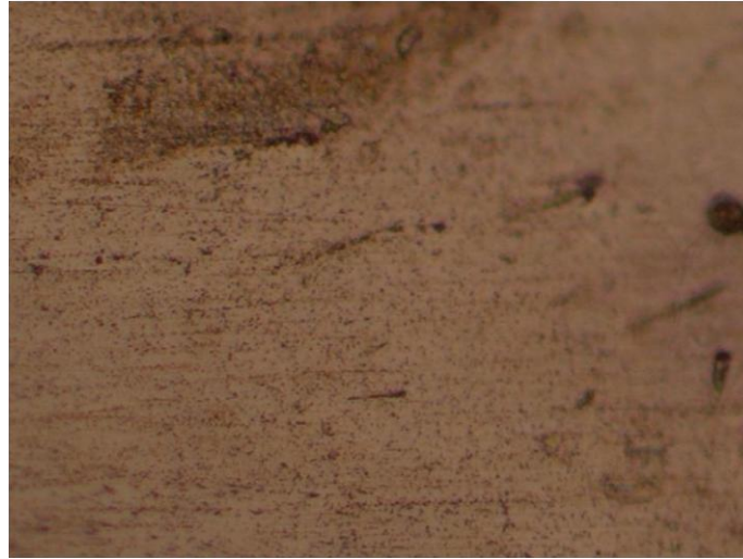
Figure 28 Microstructural aluminium 3003 FAZ and SZ Keller's reagent 200x
