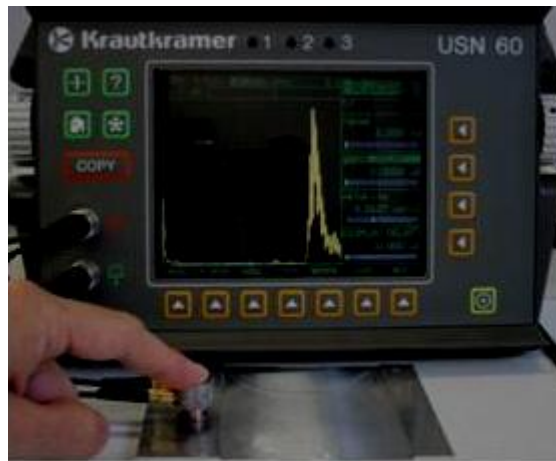
Figure 48 First calibration into the kraufkramer
