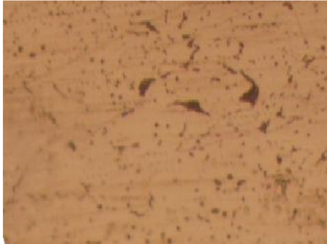
Figure 26 Microstructural aluminium 3003 TMAZ Keller's reagent 200x
