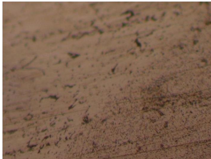
Figure 25 Microstructural aluminium 3003 SZ and TMAZ Keller's reagent 200x
