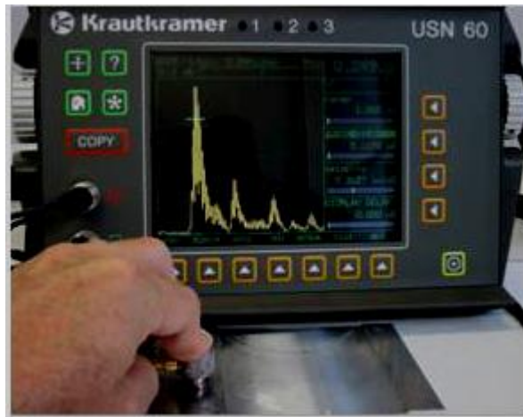
Figure 49 Calibration of time delay
