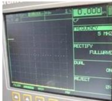
Figure 47 Receiver submenu of krautkramer
