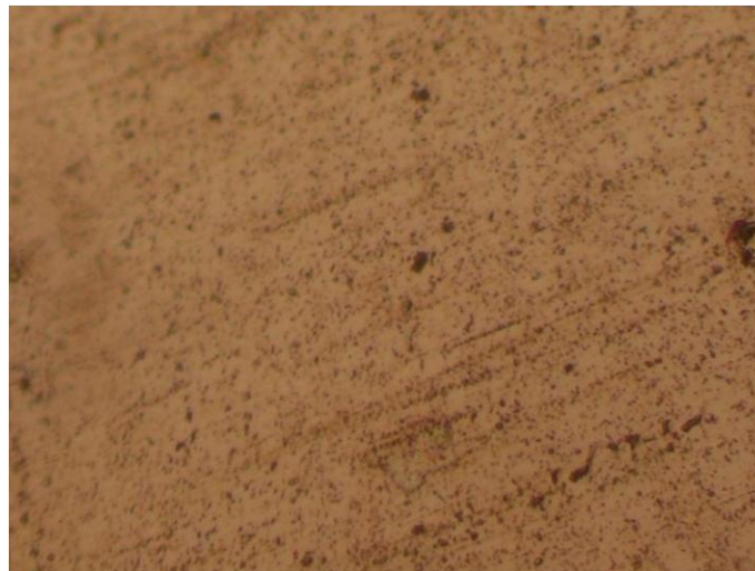
Figure 27 Microstructural aluminium 3003 SZ Keller's reagent 200x
