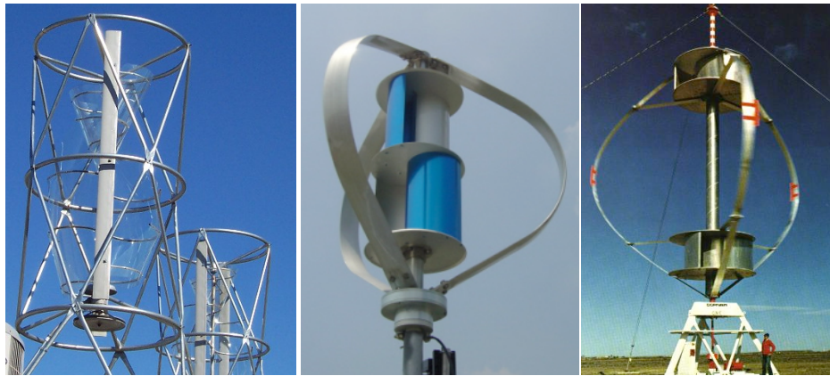
Figure 12. Combination of Savonius-Darrieus rotors, Becker at left and traditional combination at center and right. [generated by the author according to different internet sources]
