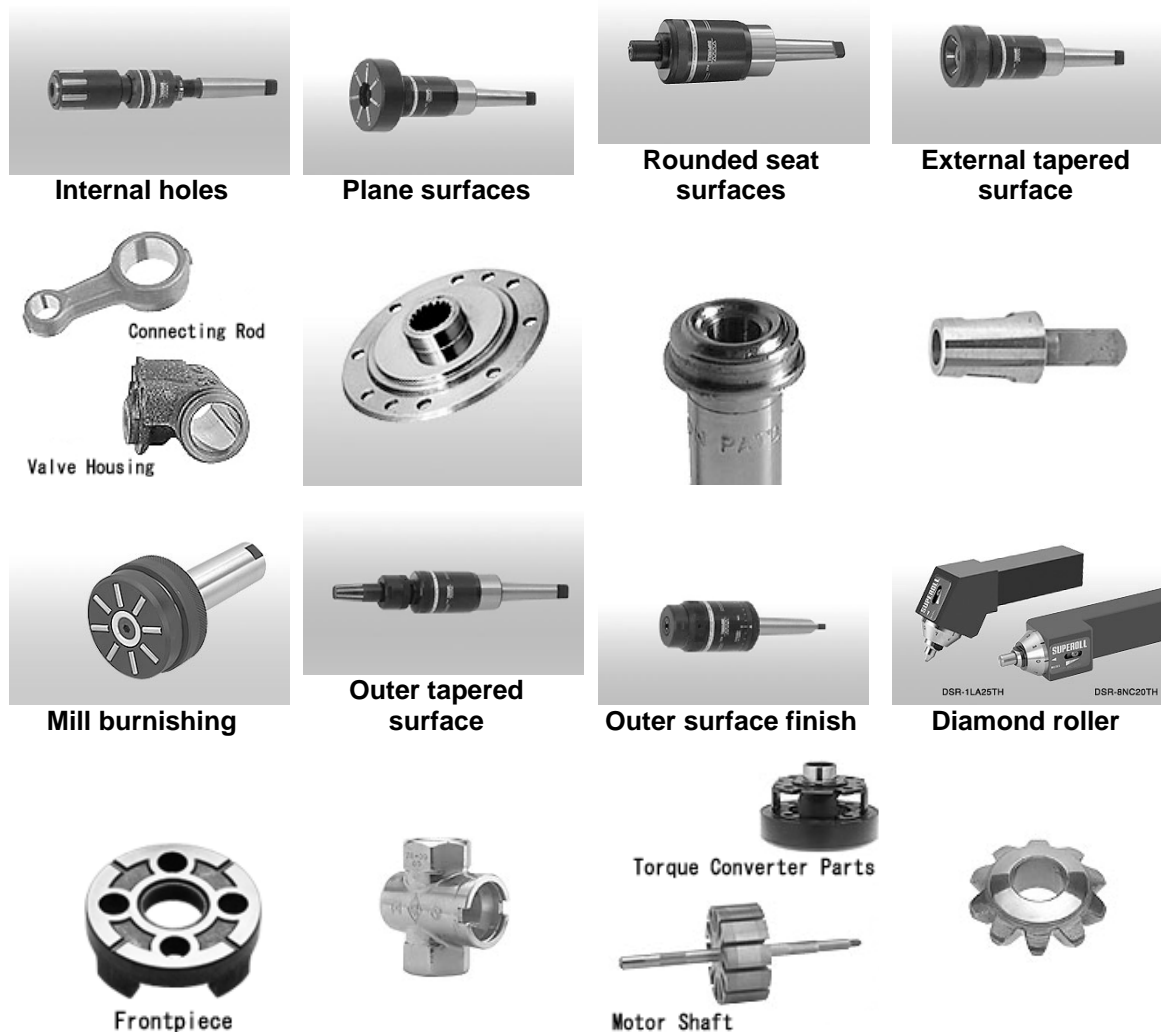
Figure C-1: Spring-loaded roller burnishing tools and some industrial applications [Sugino, 2004].
