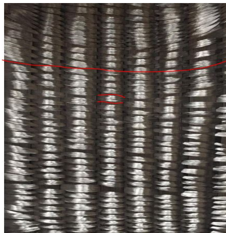
Figure 5.1: Over tension of weft yarns
