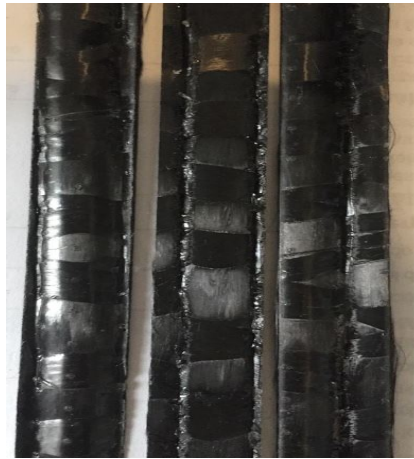
Figure 5.2: 3D woven composites VaRTM defects.
