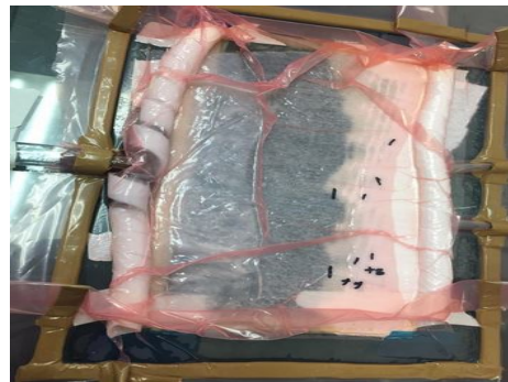
(b) Resin impregnation by RI process.
