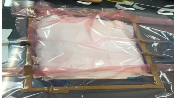
Figure B.5: Vacuum bag positioning.
