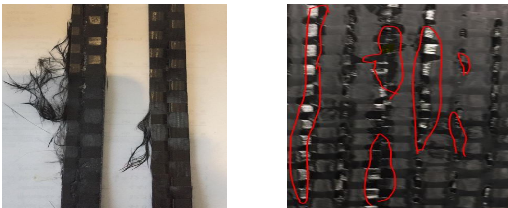
Figure 5.3: 3D woven composites Mold A defects.
