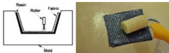
Figure 2.8: Hand lay-up Process [65].
