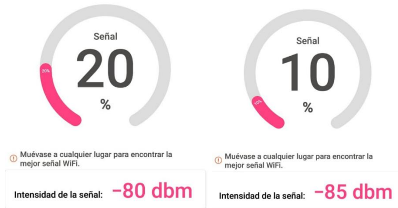
Figure C-4. Maximum and minimum signal level at a distance of 60 meters with NLOS.
