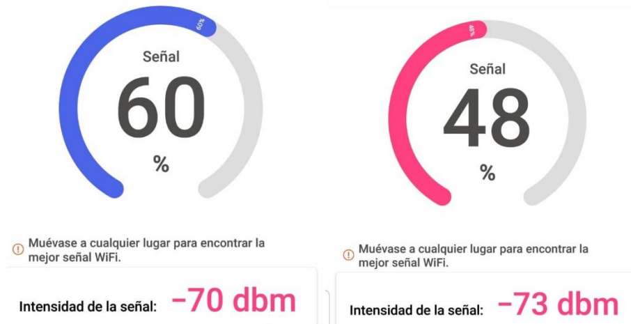
Figure C-2. Maximum and minimum signal level at a distance of 50 meters with NLOS.
