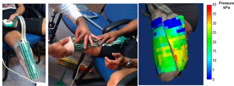
Figure 7. Example of implementation of acquisition systems for interfacial pressure measurement and color pressure mapping (figures from [25], [26]).
