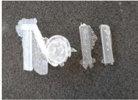
Figure 57. Ultrasonic injected Microneedle pieces. From left to right SLM insert, SLM insert and DLP insert
