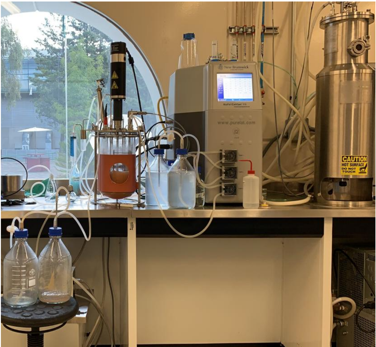
Figure 6: Bioreactor system (BioFlo Celli/Gen 115 New Brunswick Bioreactor) used to established the continuous culture of Xanthophyllomyces dendrorhous
