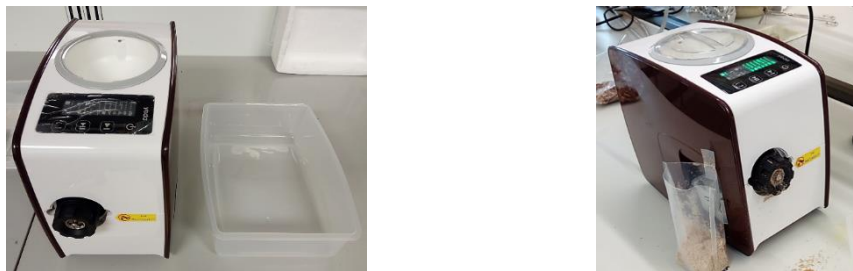
Figure 3.3 Screw pressing machine used to oil extraction from fresh and dry kernels pretreated by PEF.
