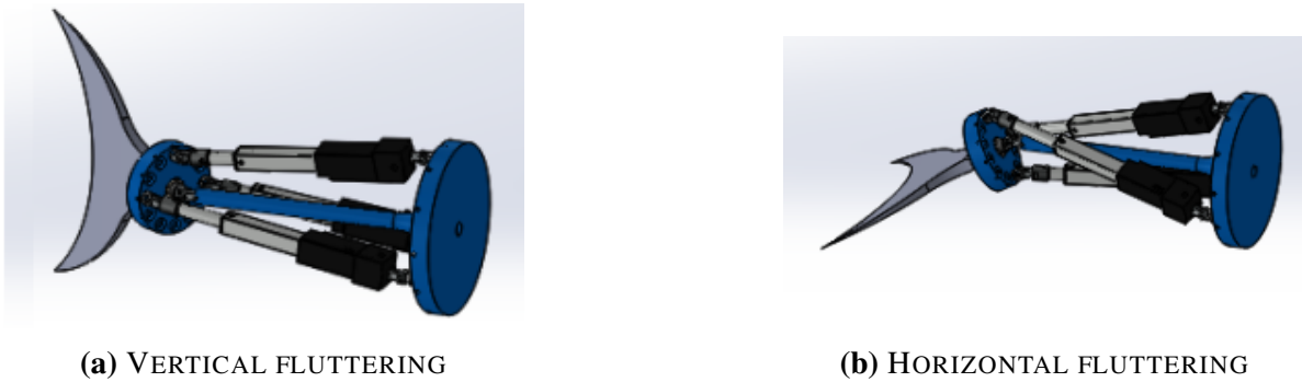
Figure 3.4. POSITIONS OF THE CAUDAL FIN FOR MOTION
