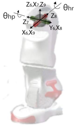
Figure 3.4: Forward orientation analysis of the humanoid leg
