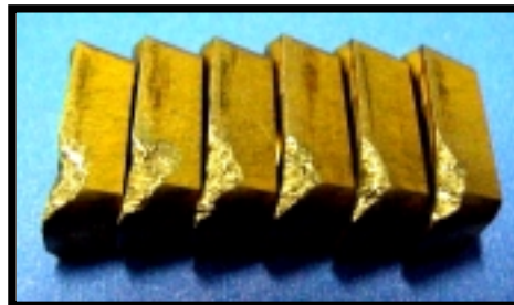
FIGURE 6. INSERTS FAILURE IN INSERT A (REMOVED MATERIAL, MR=10.5 IN 3 )
