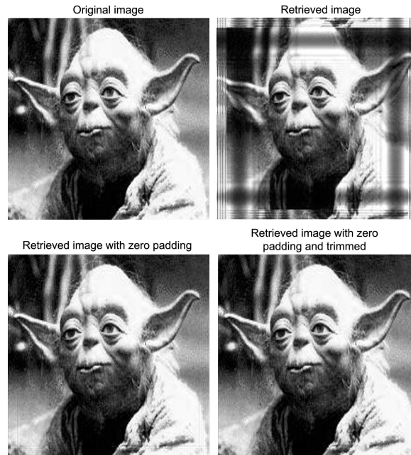
Figure 8: Results of image retrieval with the fractional Fourier transform.
