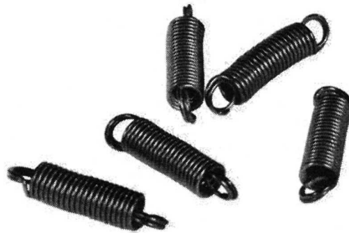
Fig. 1-1. NiTi springs in their original shape (Grand-Illusions, 2011)
