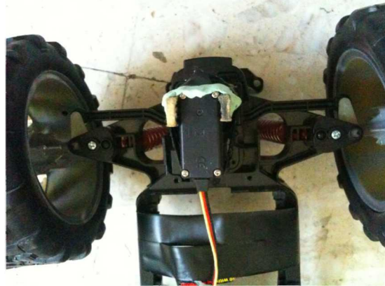
Figure 15: Servomotor attached to the steering system.
