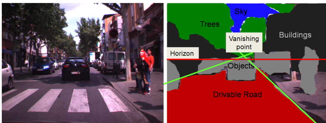
Figure 5: Detection of the horizon line according to [3].
