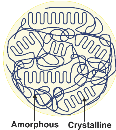
Figure 6. Illustration of UHMWPE powder crystallites embedded in a disordered and entangled chain network.
