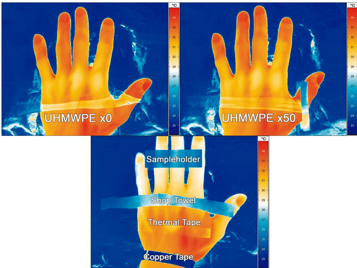
Figure 11. Thermography of UHMWPE x0 and x50 films and other materials to demonstrate the IR transparency of UHMWPE films obtained by IR Camera InfraTec 9500.
